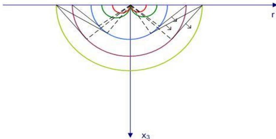
Geometry of waves in nonlocal model: two Rayleigh's (red, green), three cone waves (with arrows), mechanical transversal wave (blue), coupled thermal wave (violet), coupled longitudinal wave (light green).
